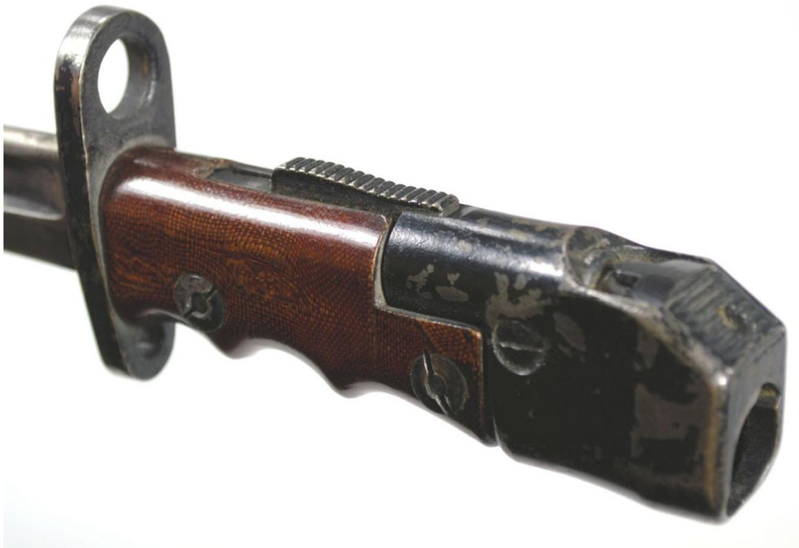
As the project developed, the incorporation of a flash-hider in the crossguard became a final element of what became officially designated Bayonet No.10 Mk.1, for use with the Enfield Model 2 (E.M.2) rifle.
