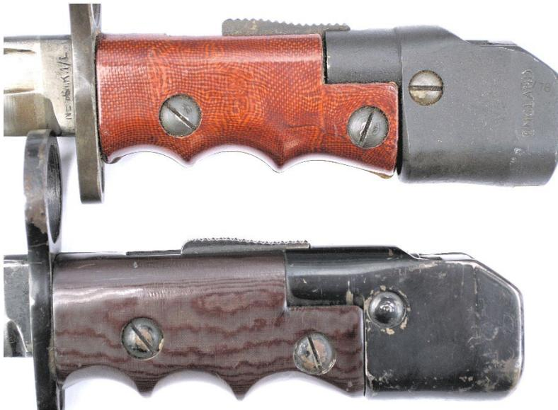
Other differences are more subtle. Nevertheless, they set the Wilkinson (bottom) apart from regular production bayonets. The socket locking pin is a bolt, not a slot head screw.
