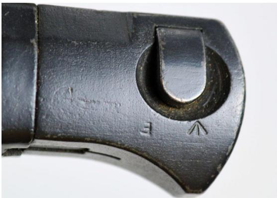
L1A1 bayonets were upgraded by milling a recess in the pommel and reducing the press stud so that it was flush.
