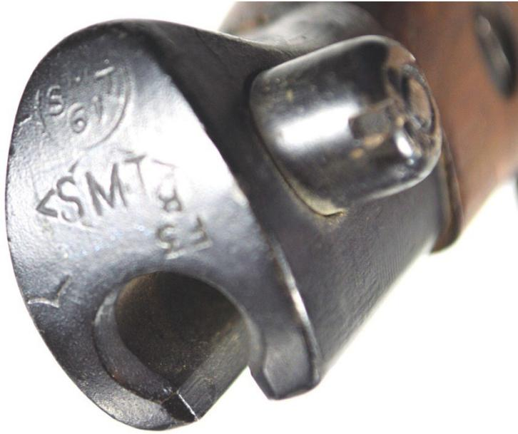
The pommel casting was sub-contracted to the Scottish Motor Traction Co., and stamped accordingly on the end S.M.T. within a diamond.
