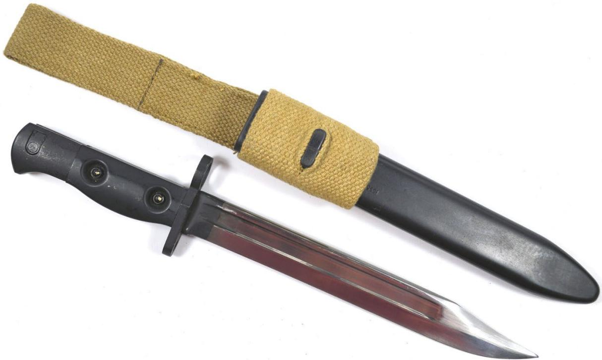
The differences from the L1A3 lay mainly in manufacturing and assembly variances. The L1A4 was produced by Hopkinson Ltd. of Sheffield in the early 70s and their logo and year of manufacture can be found stamped into the blade.
