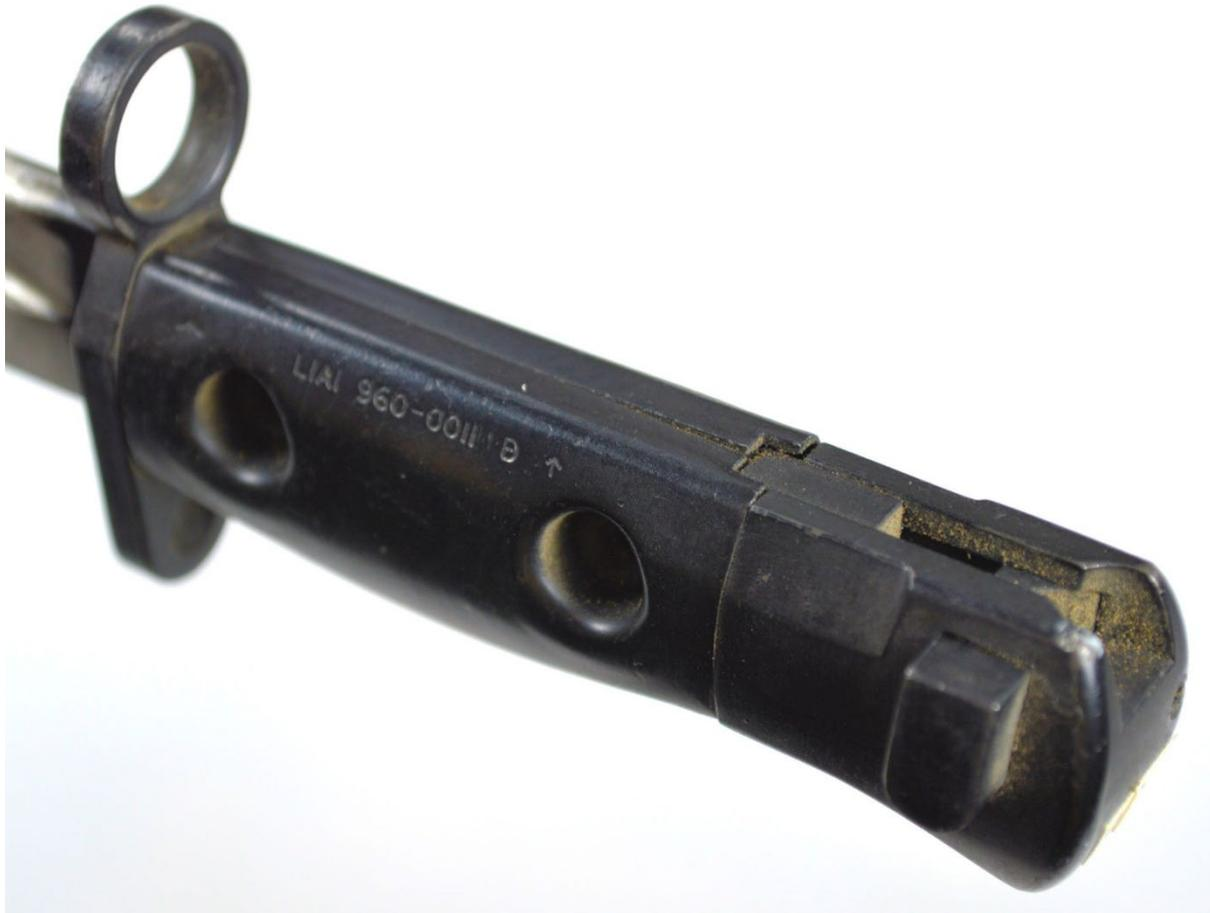
The bayonet hilt was fitted with steel grips that were impressed with the designation L1A1, the NATO stores number 960-0011 alongside a Broad Arrow.
