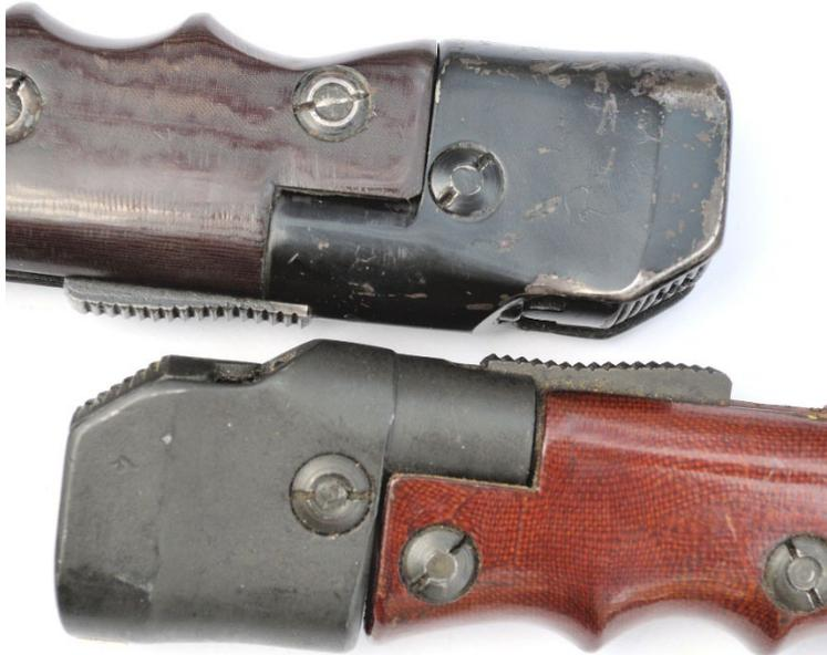
Finally, the casting of the socket on the Wilkinson is smooth, compared with production bayonets, which display a distinct ridge.
