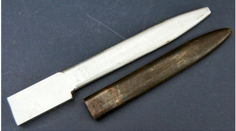
This particular item is an aluminium casting, for ensuring that L1 scabbard bodies are within the measurement tolerances set out for their production.
