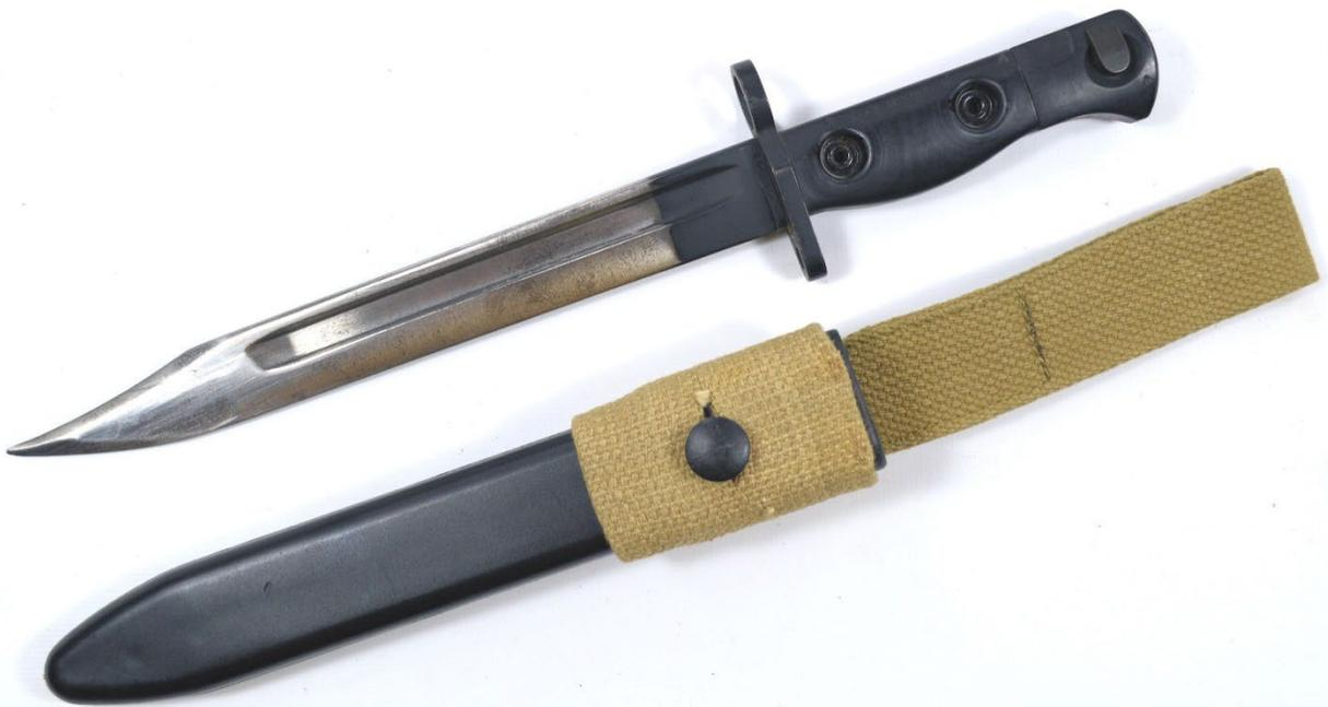
A further version of the L1A3 bayonet was produced in the mid-1960s. The long fuller was found to create a weakness in the blade and make tempering problematic. The fuller was shortened, and a new crossguard with straight sides applied by brazing to the tang, rather than riveted.
